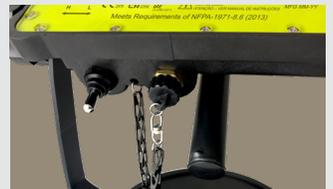
Sealed switch and charging port cap ensure full IP-67 waterproof & dust-proof protection.
